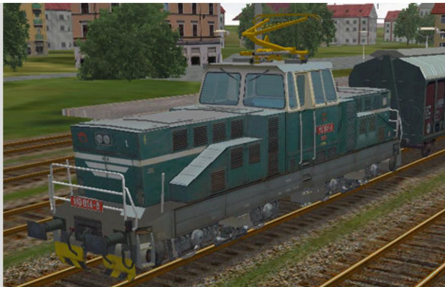
Electric shunter also used for trip freight work, and some passenger work. The 111 have chopper control.
