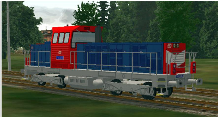
The 714 are 29 Locomotives rebuilt from retired class 735 with new Skoda motors (Some are 600kw and 90 km/h). The 714.2 have a lighter axel load. Both have electronic braking
