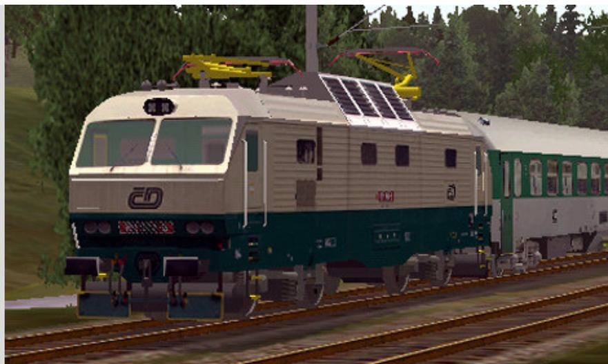
A 3kV DC Bo-Bo locomotive used for fast passenger services. The entire class will be rebuilt as Class151 for 160 km/h.
