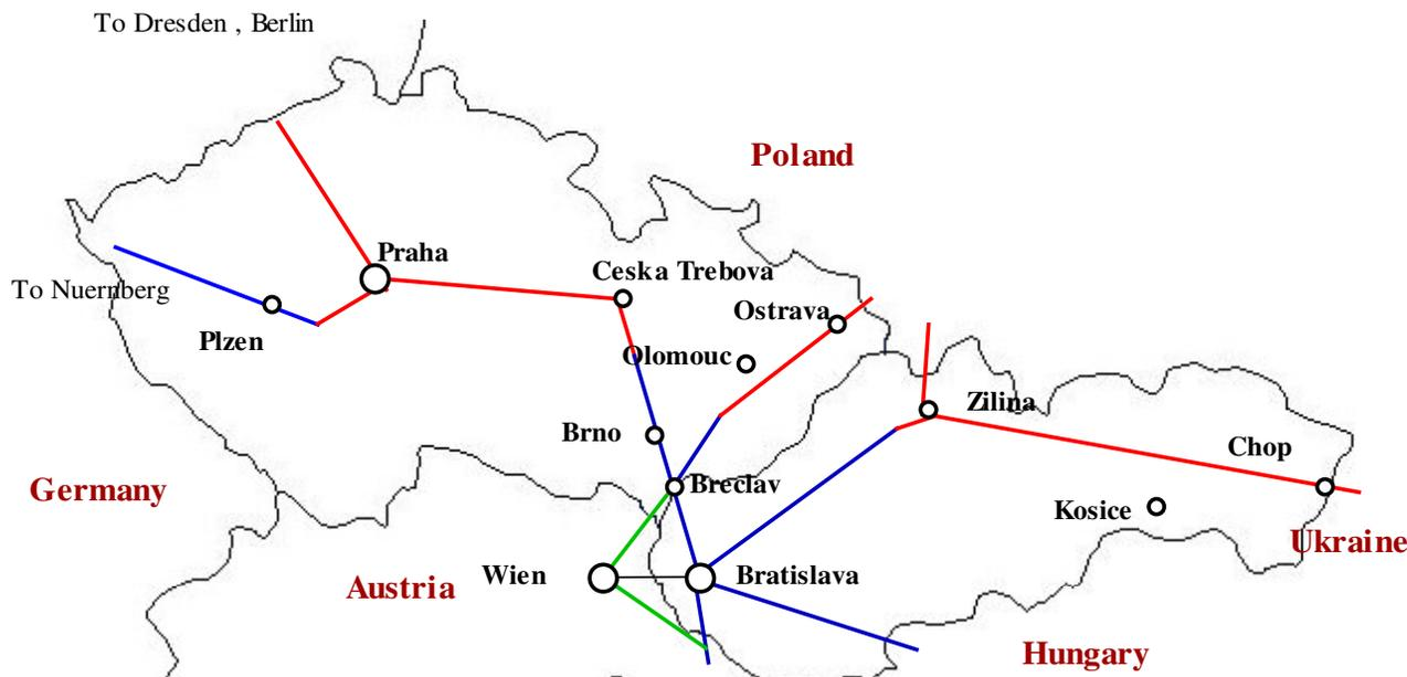
A highly schematic map showing the Trans European Network (TEN) corridors going through Czechia and Slovakia. Blue is electrified at 25kV 25Hz AC, Red 3000 V DC. Green is 15kV AC 16.7 Hz.
