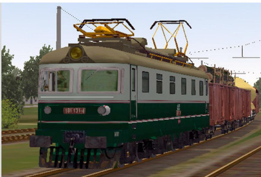
A 3kV DC Co-Co locomotive used for heavy freight duties capable of pulling 50 tonnes of freight cars as 90 km/hr. The 180 was the prototype
