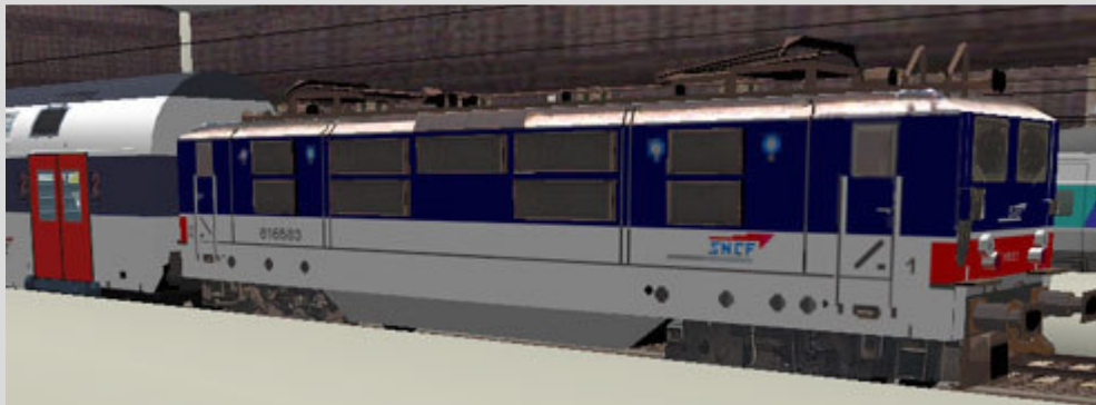
A BB 16500 in Ile de France livery with Double-deck push-pull VB2N stock Model: Jean-Pierre Gleonec
