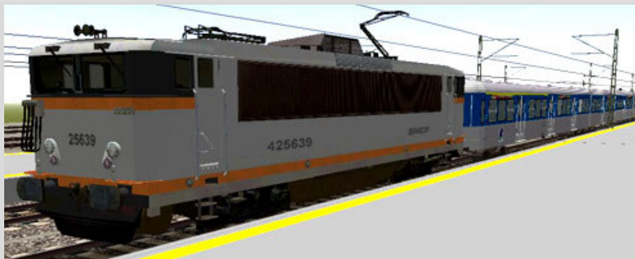
A BB 25600 in Béton scheme equipped for push-pull with a RIO trainset Antibes (PACA) July 1999 Model: Serge Carrey
