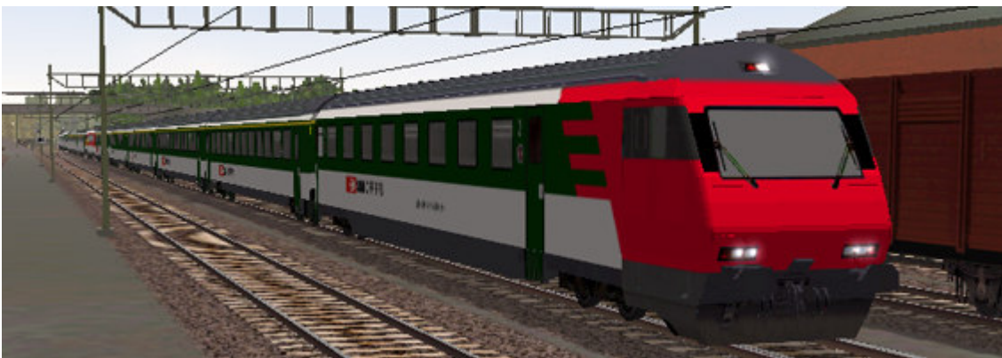
The EW IV Driving cab with the front based on the Re460, in the original White/green livery. On Zurich to Geneva trains the driving cab is at the Geneva end. Model Hayo Schelten
